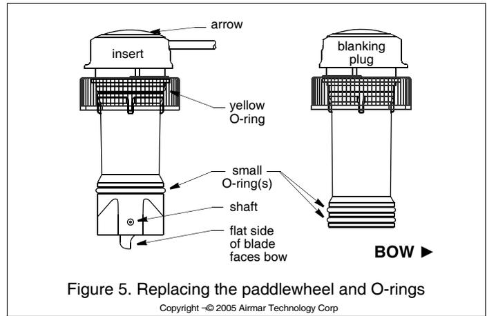
The water lubricated paddlewheel bearings have a life of up to 5 years on low-speed boats [less than 10kn (11MPH)] and 1 year on high-speed vessels. Paddlewheels can fracture and shafts can bend due to impact with water borne objects and mishandling in boat yards. O-rings must be free of abrasions and cuts to ensure a watertight seal. Order a replacement Paddlewheel Kit No. 33-540-01.
